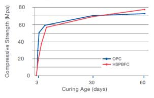
Compressive Strength Development of Typical OPC and HSPBFC Concrete The correct fineness of the OPC and GGBS particles is necessary for the concrete strength development.
